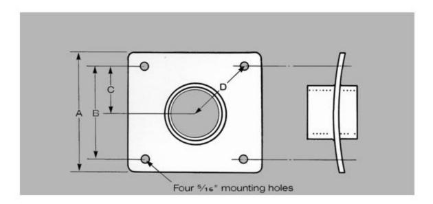
CONSTRUCTED FROM STAINLESS STEEL (RECOMMENDED FOR DISCHARGE CONNECTION). COUPLINGS INCLUDE GASKET, NUTS, BOLTS, AND WASHERS.
